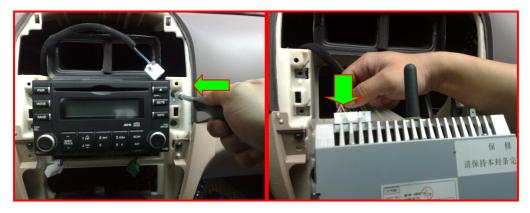
4. Connect the special cables, then install the screws of the bracket.
