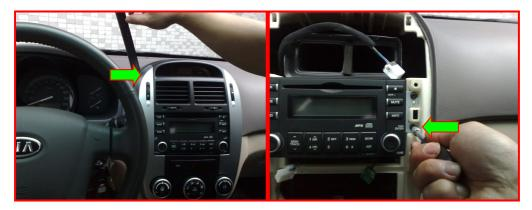
3. Take out the attaching plug afer loosen the screws.
