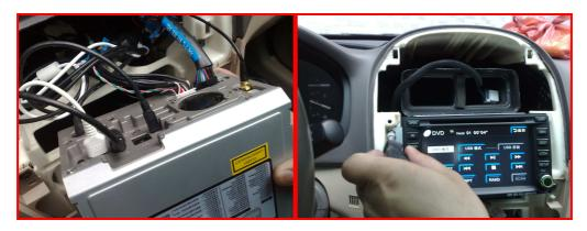
6,Connect the climate cable well,then install the console pane back well.
