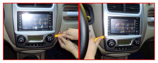
3. Take out the console panel lightly, then loosen the screws of the main unitl
