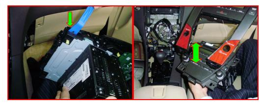
8. The 6CDC fixing in the FLYAUDIO main unit, then fixing the screws of the bracket.
