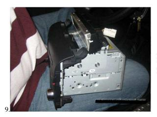
Add the brackets in the device for both sides and put together the little LCD with the new device.
