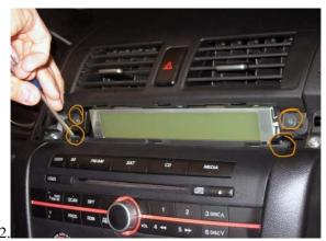
Remove the 4 screws holding in the vents and stock head unit.
