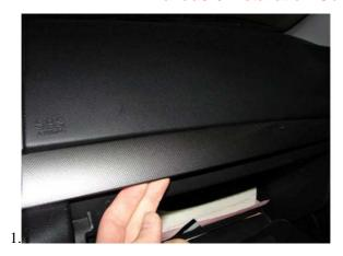
Start by opening the glove box and removing the trim but lifting from the middle to the left and the last part to come out is the far right against the door.
