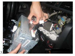
Pull the head unit out and remove the factory wire harness from the radio.
