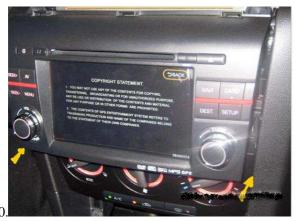
before introducing the device, make sure everything is working correctly, when its working propertly, fix all the cables in the back part, then you can put the device in from both sides at the same time.
