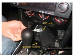
Connect the Bluetooh receiver with the device. This connection is very important because you'll be able to get the little LCD working also. Join CAN+ (device) with cable with CAN+ (Bluetooh receiver) and the CAN- (device) with CAN- (Bluetooh receiver). If not working, make a crossover: CAN- to CAN+ and CAN+ to CAN-. It should works.
