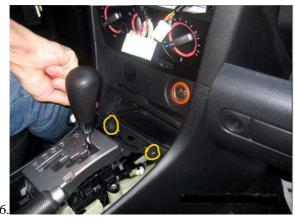
Remove the 2 screws to pull the ash tray out.
