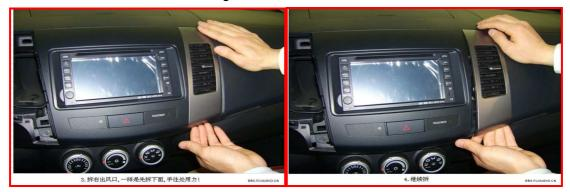
3.Remove the two screws of the console panel, then take out the inside frame first.
