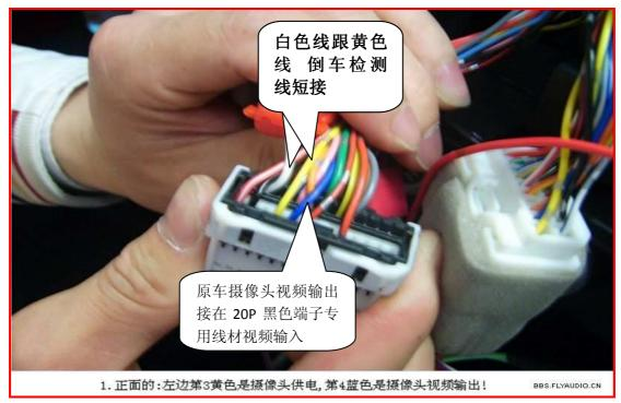
(2)From the front side: the third one which is yellow from the left is the cable for the power of the camera, the fourth one which is blue is for the output of the camera video
