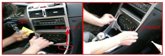
4.Remove the screws of the air-condition board, take it out with the CD module
