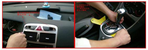
3. Prize up the console panel after remove the screws, then take out the console penel.
