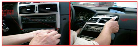
5. Take out the plug of the CD unit, then cut off the support bar of the console panel.
