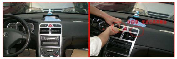
2.Remove the fixed screws of the air-condition board, prize up the gear board.
