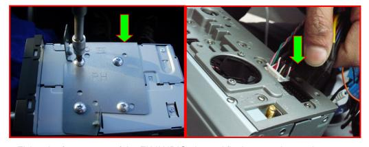
4. Fixing the four screws of the FLYAUDIO uint, and fix the console panel.
