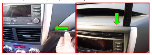
2.Remove the screws of the original main unit and connect the special cables.
