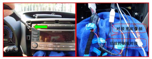
3. Fit the original brackets at the FLYAUDIO unit, and connect the cables to the back side.
