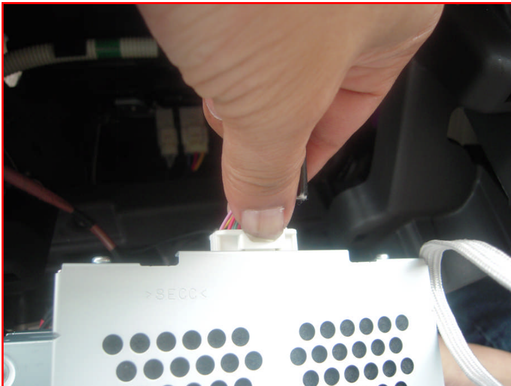
32: Connect the connectors to the factory screen
