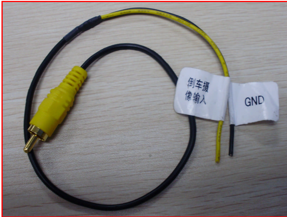
27: The cable used to connect the original camera
